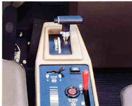
K-ATOMiCS (Komatsu Advanced Transmission with Optimum Modulation Control System)
